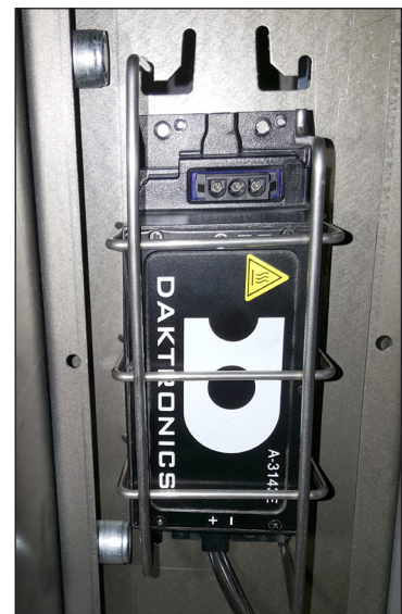
Figure 22: Power Supply Mounting
